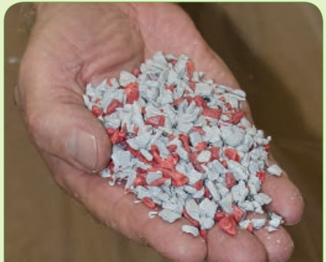
AGS’s proprietary Injectoblend materials are tightly specified salt-and-pepper blends of scrap regrind and additive masterbatches. AGS has developed techniques for molding these blends without repelletizing.
