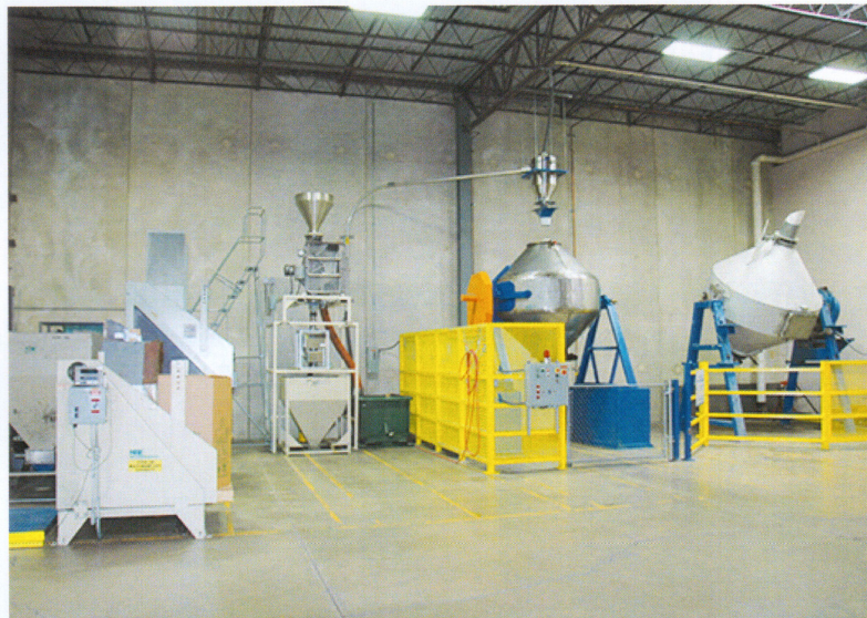
Inside AGS' facility, you will not find typical equipment configurations. Equipment includes gaylord tipplers; a cleaning, de-dusting, metal separation module; and two double-cone
